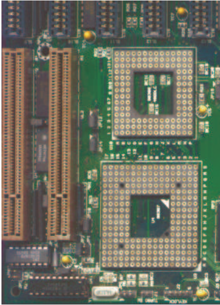
Vesa Local bus slots (brown) below the ISA slots on a 386/486 motherboard.
